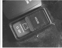
**NOTE:** The combination carbon monoxide/propane alarm must be connected to a constant 12-volt power source. The carbon monoxide/propane alarm remains operational when the battery disconnect solenoid switch, or “main power switch,” is in the “off” position.
